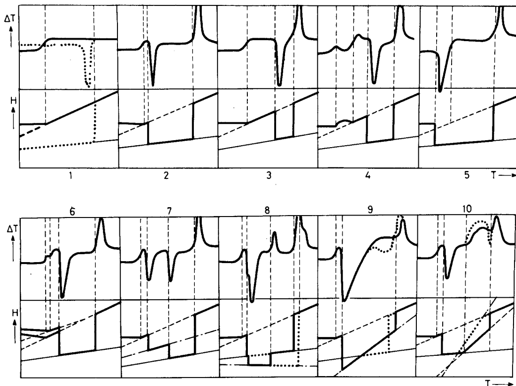
Fig. 2 Hypothetical enthalpy ( H ) plots (lower) and corresponding DTA curves ( \Delta T ) for some characteristic cases that may be met during investigation of a glass upon reheating. Temperatures specific for individual changes indicated on the \Delta T vs. T plots are marked by verticals.
